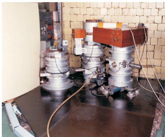
Fig. 2(a) Photograph of the QENS spectrometer installed at beam tube TT1004 at DHRUVA
