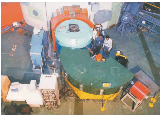
Fig. 1 The upgraded version of the High-Q diffractometer showing Monochromator drum, Sample table and the Detector shield assembly.
