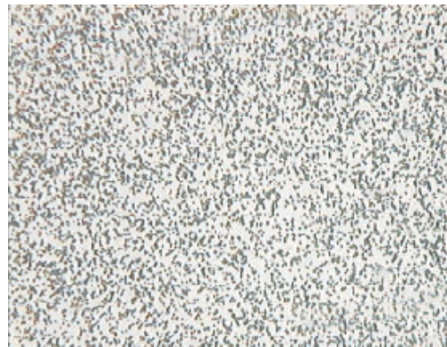
Fig. 8 Alpha Autoradiograph of a MOX fuel pellet showing uniform distribution of Plutonium in the matrix
