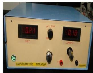
The performance of the instrument has been tested with actual experimental solutions in lab and the results were in good agreement with existing analogue instrument. In the analogue instrument, the end point was seen in  $\mu\text{A}$  current range, but with the digital instrument, the end point is seen up to nA current range. Detail studies and further improvisation are in progress.
