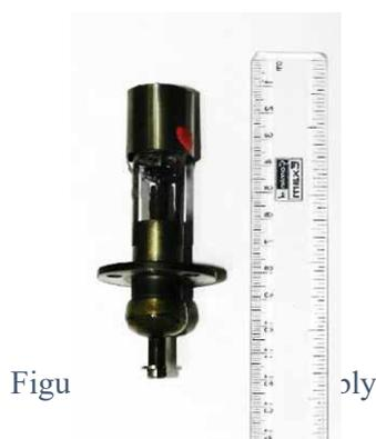
Figure 1: Photograph of the cathode assembly.
