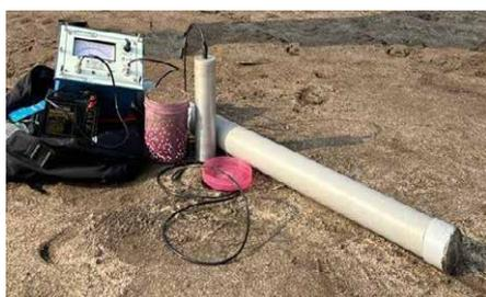
Fig. 1. NaI (Tl) detector connected to the count rate
