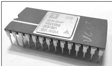
Fig. 1: An ASIC 28 Pin DIP VECC003
