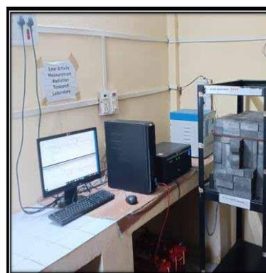
Fig.1. 4"X4" NaI(Tl) scintillation detector based gamma ray spectrometer
